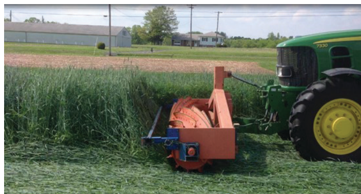
Figure 1. The roller-crimper rolling down a cereal rye cover crop in a no-till field.
