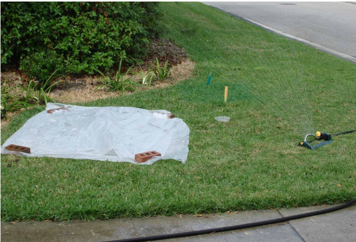
Figure 3. More irrigation is applied to the second treatment area so that it receives a higher amount of irrigation, while the first area is covered with the tarp so that it receives a lower amount of irrigation.
