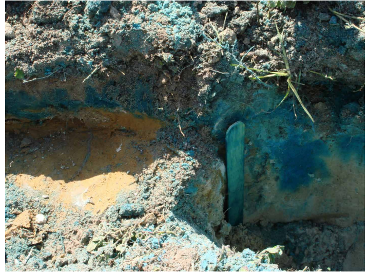
Figure 5. This photo shows a comparison of the depth that the dye moves in clay soils (left) versus sandy soil (right).
