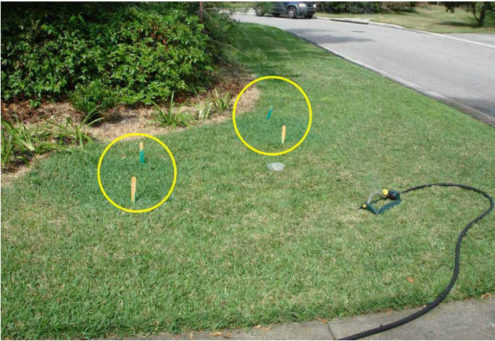
Figure 2. Irrigation is applied to the turf after dye was applied to two areas (each 3 sq ft) marked by the stakes. Notice that a container is catching the irrigation water to measure the amount of irrigation applied.
