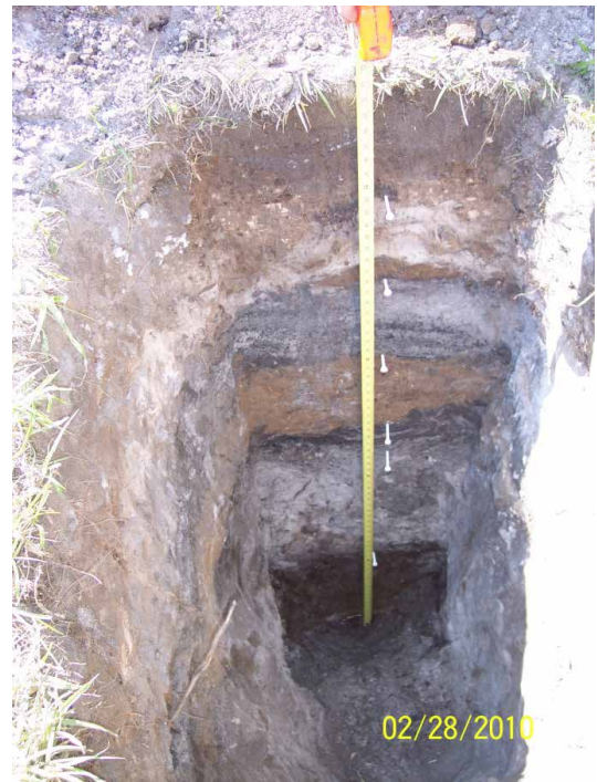
Figure 2. Fill sand is typically added to a construction site to raise the elevation, resulting in the burial of the native soil profile. In this picture, note that various fill materials were applied in layers to establish the final grade. Credits: Don Rainey
