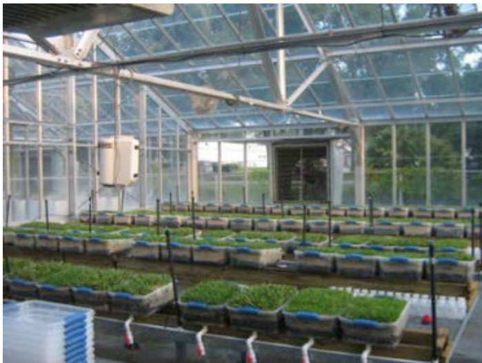
Figure 1. Overview of greenhouse set-up, showing the growing tubs with established sod and the drains for collecting leachate. Credits: Dr. Jinghua Fan
