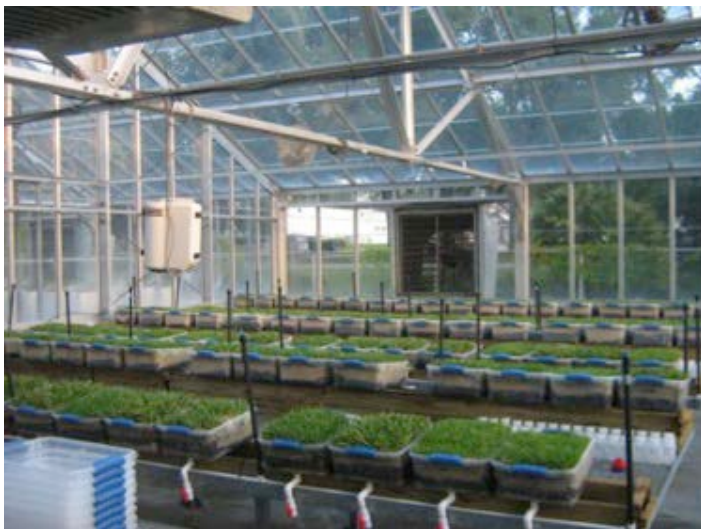
Figure 1. The overview of greenhouse operation showing the growing tubs with the established sod and the drains for collecting leachate. Credits: Dr. Jinghua Fan
