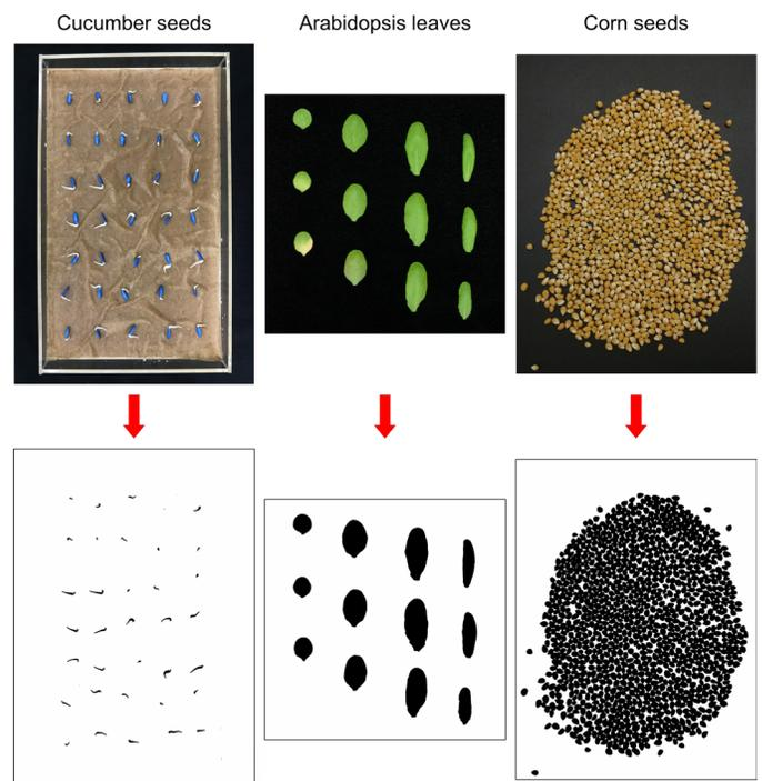
Figure 1. Conversion of color images to binary images for automatic counting using ImageJ (not to scale). In the leaf image, leaf area can also be measured simultaneously.
