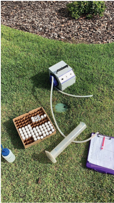
Figure 11. Equipment and supplies for leachate sample collection, including battery-powered peristaltic pump, graduated collection container, rinse bottle with deionized water for decontamination, sample collection bottles, and field sheet for recording leachate volumes.
