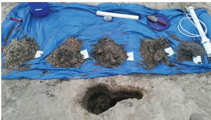
Figure 4. Each lift of soil is placed separately on a tarp and labeled to rebuild the soil profile later. Credits: Eban Z. Bean, UF/IFAS
