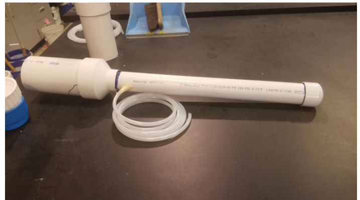
Figure 2. Assembled drainage lysimeter with collection chamber, reducer, reservoir, and purge tube shown. Credits: Jovana Radovanovic, UF/IFAS
