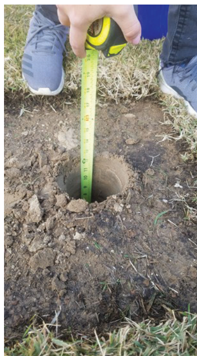
Figure 3. Measure and record the depth after excavating each lift of soil.
