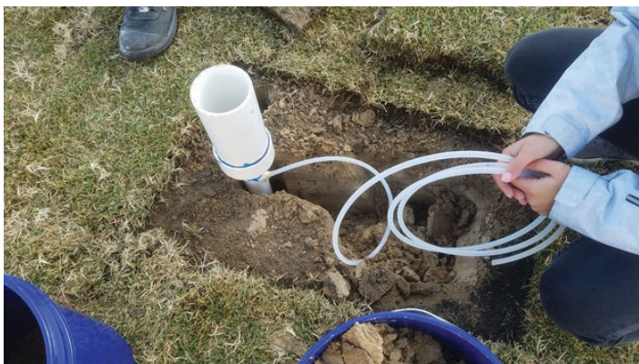
Figure 5. A notch for the collection tube is made and the lysimeter is ready for pea gravel. Credits: Jovana Radovanovic, UF/IFAS
