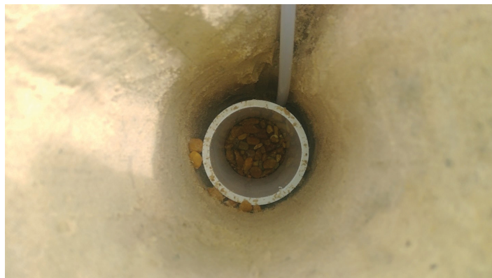
Figure 6. View of lysimeter from soil surface after adding pea gravel onto the mesh screen.
