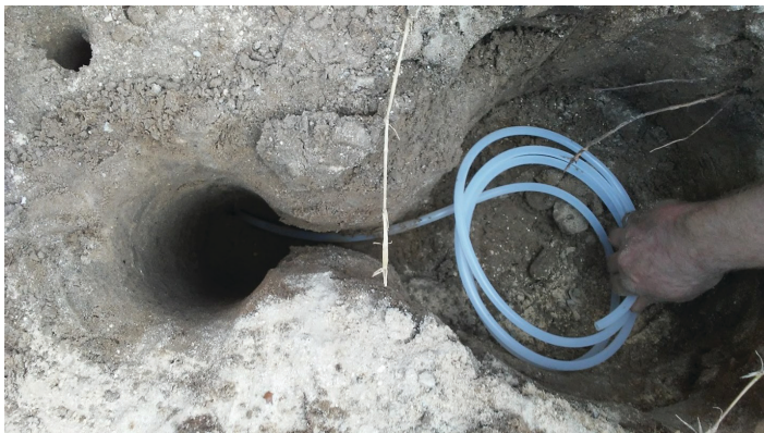
Figure 8. Excavate a void adjacent to the lysimeter cavity to store the leachate sampling tube and tube housing. Credits: Jovana Radovanovic, UF/IFAS
