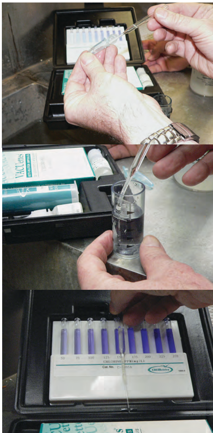
Monitoring dump tank water chlorine levels manually
