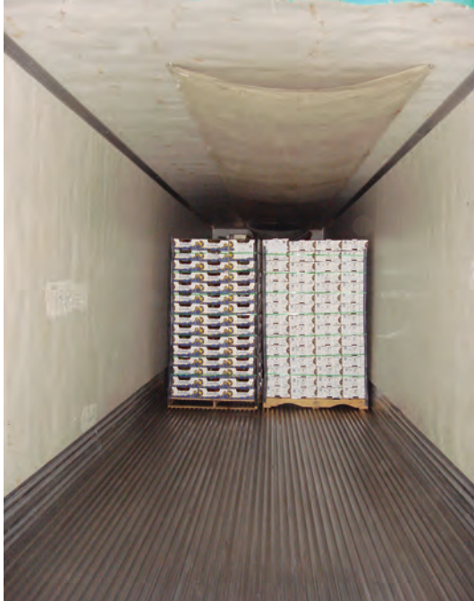
Inside of a trailer being loaded; the air delivery chute is shown
