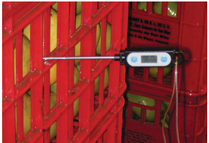
Measuring mango flesh temperature following hydrocooling
