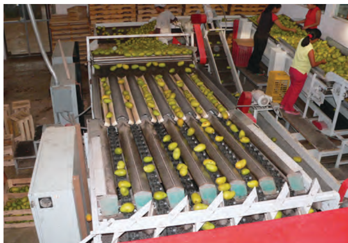
Automated fruit sizing on the packingline
