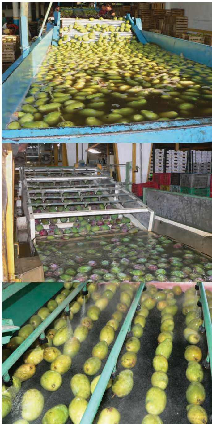
Initial fruit washing by tank immersion (top), spraying (middle), and on a brush bed (bottom)
