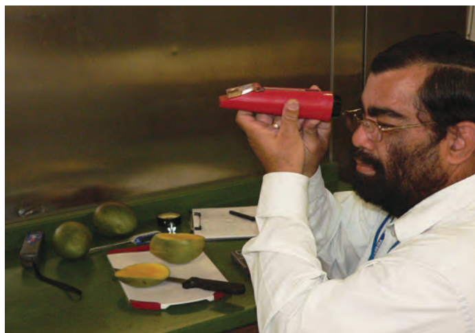
Measuring mango fruit TSS with a refractometer
