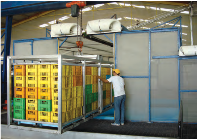
Post-hot-water treatment hydrocooling
