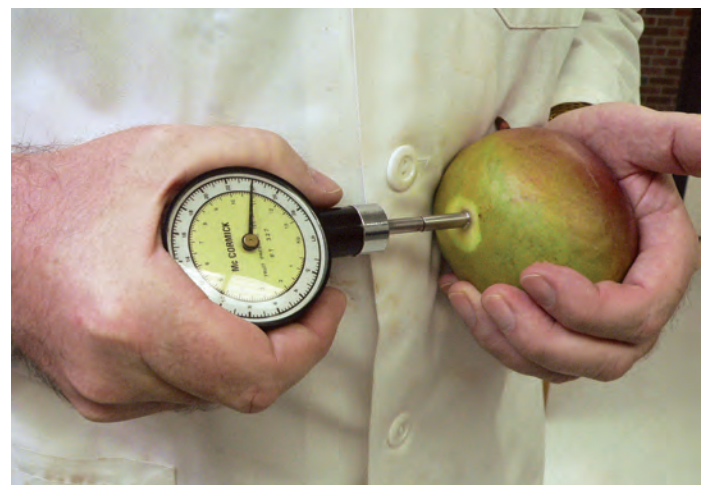
Measuring mango flesh firmness with a penetrometer
