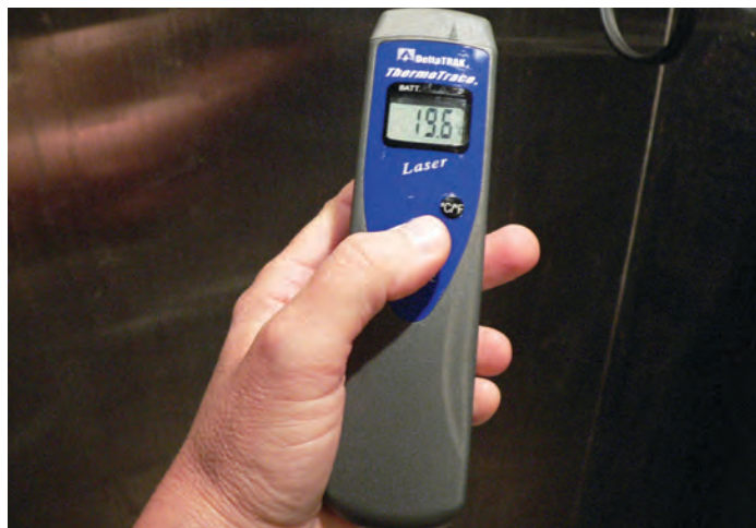
Measuring surface temperature with an infrared thermometer
