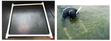
Figure 3. Examples of quadrats. This quadrat is made of  $\frac{34''}{1000}$  PVC. Note that the corners have holes that allow water to flow into the pipe, causing the quadrat to sink. This quadrat is 0.5 m × 0.5 m, so counts would be multiplied by 4 (or divided by 0.25) to get total counts per m<sup>2</sup>.
