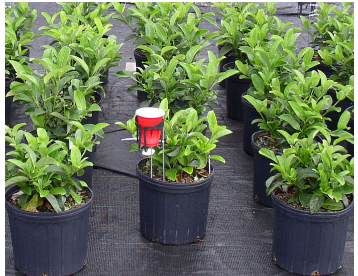
Figure 6. Reservoirs are used to monitor the irrigation application amount. Credits: Tom Yeager
