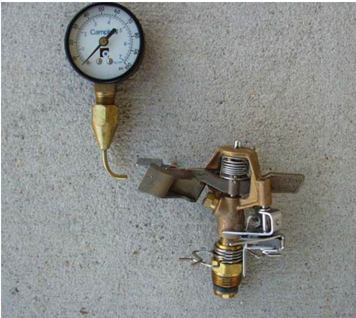
Figure 4. A pitot tube with pressure gauge is used to monitor pressure as water flows from the orifice. Credits: Tom Yeager
