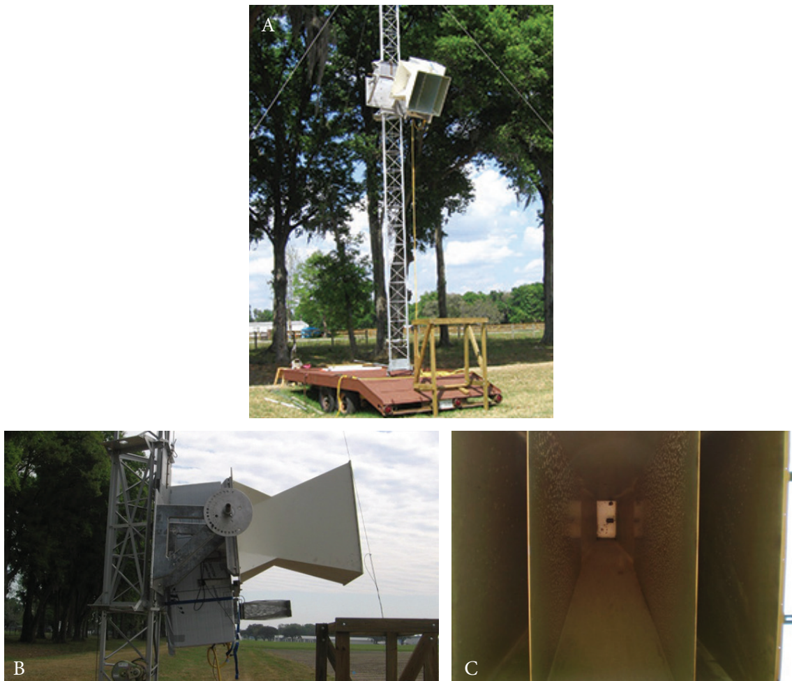
Figure 6. (a) The UFLMR system, (b) the side view of the UFLMR showing the rotary system, and (c) the front view of the UFLMR showing the receiver antenna.
