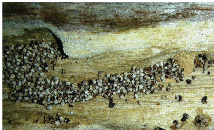
Figure 8. The galleries of drywood termites are excavated through the wood regardless of grain. The walls of the galleries are clean with dry loose fecal pellets.
