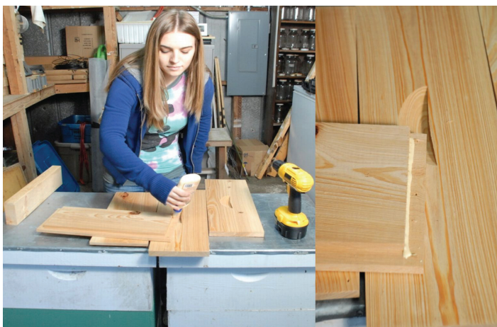
Figure 2. Wood glue should be applied in sufficient amounts before assembling boards with screws.
