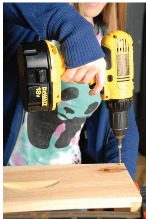
Figure 1. Using screws rather than nails helps keep the box sealed tight during expansion and contraction of the wood.
