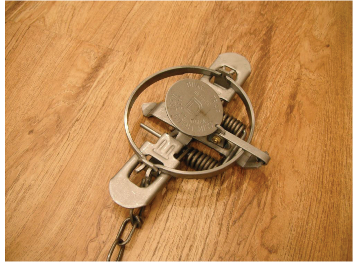
Figure 4. A leg-hold trap for catching mammals. Only traps commercially manufactured with padded jaws can be used in Florida. Credits: Holly Ober
