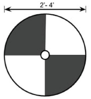
Figure 2. Schematic of a PVC/painted plywood target that can be placed at geolocation corners before every flight. Credits: Aditya Singh, UF/IFAS
