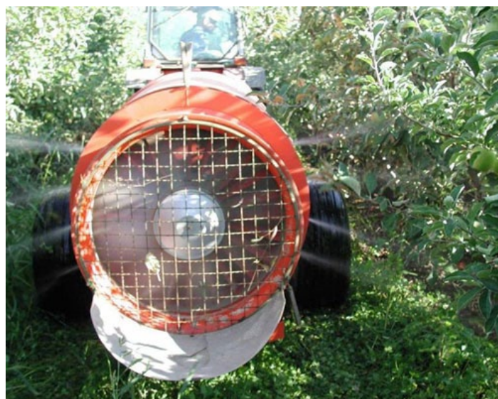
Figure 6. Applying entomopathogenic nematodes in an orchard using tractor-mounted airblast sprayer configured for this purpose. Credits: Lerry Lacey, USDA.
