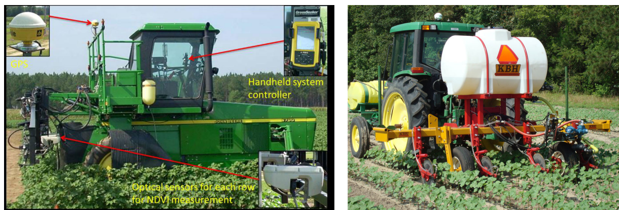
Figure 1. GreenSeeker® RT-200 integrated sensing and variable application system (left) and Clemson-designed variable-rate nitrogen applicator that does not have onboard sensors; NDVI data were collected in a previous trip across the field (right). Credits: Wesley Porter
