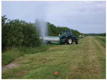
Figure 5. Airblast sprayer used to apply soluble nutrients to citrus tree foliage. Credits: P. Chris Wilson, UF/IFAS
