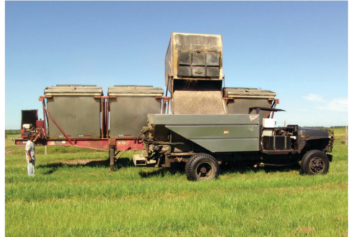
Figure 1. Unloading dry solid fertilizer from a delivery trailer to a grove spreader.
