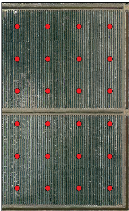
Figure 7. Example of the grid sampling strategy for selecting soil and leaf sampling locations. The red dots show predetermined sampling locations that will be recorded with GPS equipment and used to construct variability maps.
