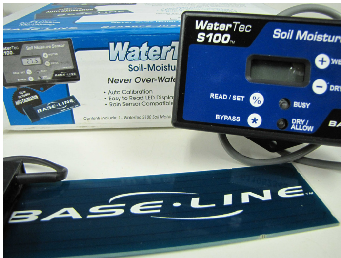
Figure 7. Example of a time-based controller with a soil moisture sensor. Credits: S. Michael Gutiérrez, UF/IFAS
