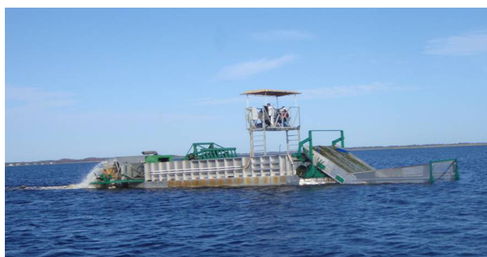
Figure 8. Mechanical harvester in the process of harvesting hydrilla.
