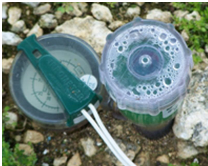
Figure 3. Tensiometer installed in very gravelly loam soil.
