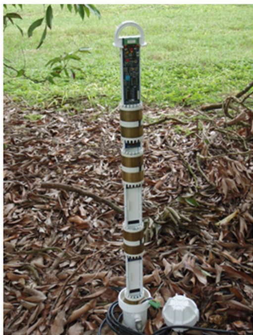
Figure 4. Multi-sensor capacitance probe being inserted into field.
