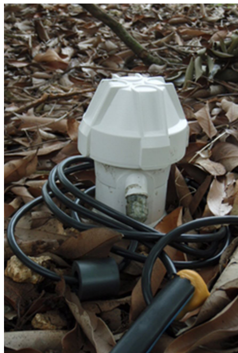
Figure 5. Multi-sensor capacitance probe installed in a south Florida grove.
