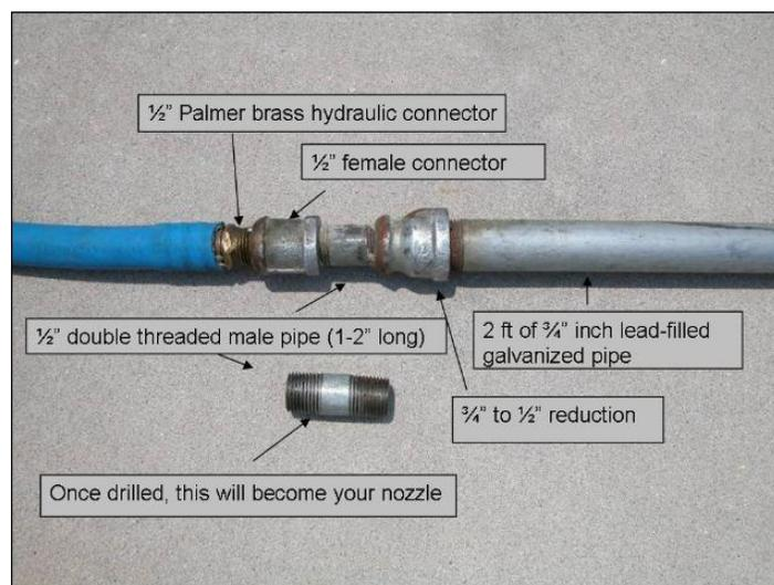
Figure 6. Trailing hose attached to the  $\frac{3}{4}$ " drilled nozzle and followed by 2 feet of  $\frac{3}{4}$ " lead-filled pipe.
