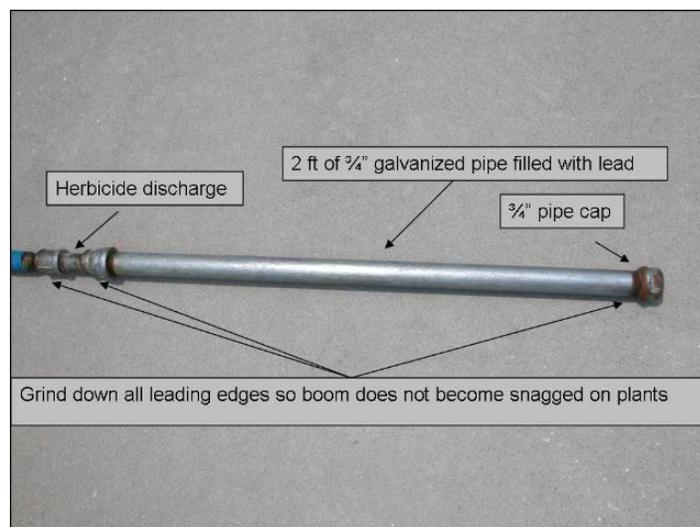
Figure 7. Lead-filled pipe at the end of the trailing hose. The depth of the lead-filled pipe will depend on the water depth and hose length and is greatly influenced by speed and weed density.
