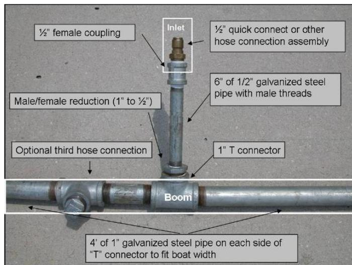
Figure 4. Inlet setup from the spray tank to the boom.
