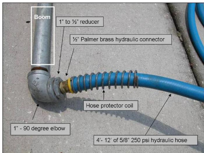
Figure 5. One-inch galvanized boom reduced to  $\frac{1}{2}$ " for attachment of the  $\frac{5}{8}$ " trailing hoses. Trailing hoses can be any length, and we use two sets for our 3-hose setup. We use three 12 foot hoses to cover the bottom acre-foot and one each of 4, 8, and 12 foot hoses to treat the total water column. To treat water that is 12–16 feet deep, use hoses that are 20–24 feet in length.
