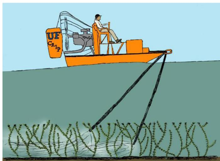
Figure 1. Bottom acre-foot treatment with weighted trailing hoses. This system delivers the herbicide directly into the weed bed for maximum efficiency and lower cost.
