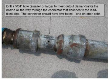
Figure 3. The nozzle for herbicide discharge can be drilled to any appropriate size. Note that the leading edges of the fitting are ground down to minimize snagging on submersed weeds. Credits: Photo by Greg Reynolds.
