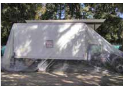
FIGURE 12 • Fumigation chamber wrapped in polyethylene sheeting.
