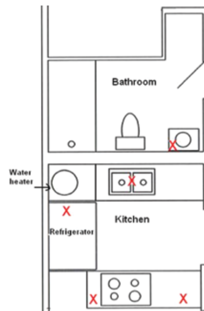
FIGURE 3 • Areas where monitors can be placed in an apartment are marked with a red “X.”
