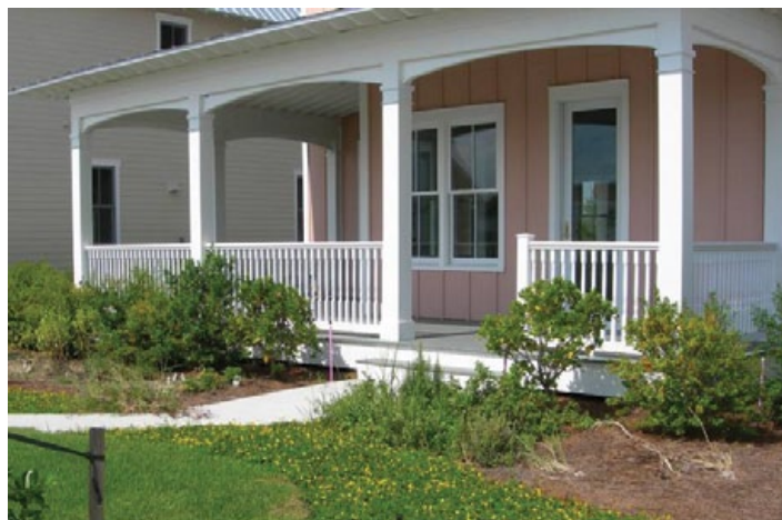
FIGURE 8. Small, fine-textured shrubs allow easy access to porch railing for maintenance.
