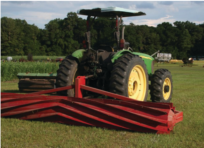
Figure 2. A ten-foot commercially available roller crimper for row crop production.
