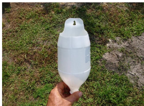
Figure 2. "Lip" to support each hanging bottle. (Credit: B. M. Santos and T. P. Salame-Donoso)
