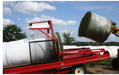
Figure 4. Round-bales of silage wrapped in an "in-line" tube.
