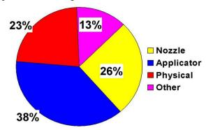
**Figure 2.** Factors contributing to pesticide drift. Credit: UF/IFAS Pesticide Information Office.
