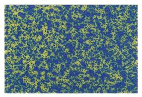
**Figure 13.** Spray coverage with an extended-range nozzle tip at 20 gallons per acre. Credit: J. A. Ferrell, UF/IFAS Dept. of Agronomy.
