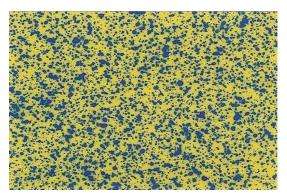
**Figure 12.** Spray coverage with an extended-range nozzle tip at 10 gallons per acre. Credit: J. A. Ferrell, UF/IFAS Dept. of Agronomy.
