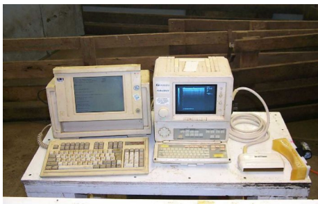
Figure 2. Real-time ultrasound machine, probe and accessories. Picture courtesy of National Pork Producers Council (NPPC) (2000).
