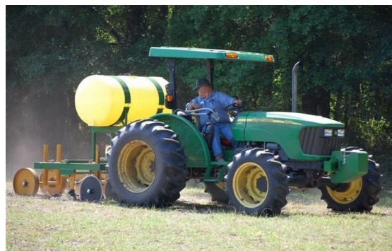
Figure 5. Nematac® S application equipment pulled behind a tractor. (Credit: UF/M.W. Warren)
