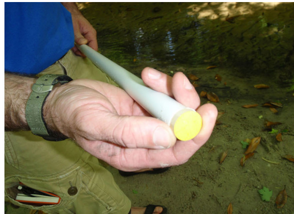
Figure 3. Mini-piezometer cap constructed from two sections of wooden dowels glued together. Photo Credit: Shantih Spanton
