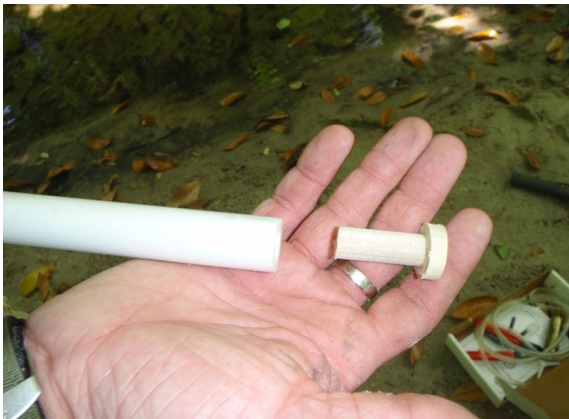
Figure 3. Mini-piezometer cap constructed from two sections of wooden dowels glued together. Photo Credit: Shantih Spanton
