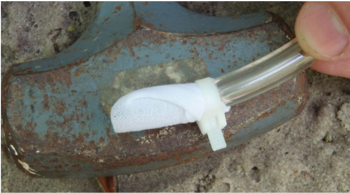
Figure 2. Nylon stocking used as filter fabric to prevent clogging of the perforations in the clear tube. Photo Credit: Shantih Spanton
