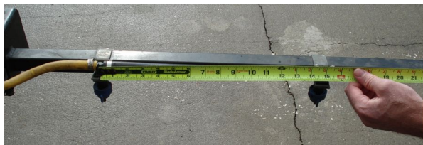
Figure 1. Measuring nozzle spacing to determine "W". Credits: J. Ferrell, IFAS/UF
