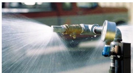
Figure 2. A wide-swath, boomless nozzle. Credits: J. Boyd - U. of Arkansas
