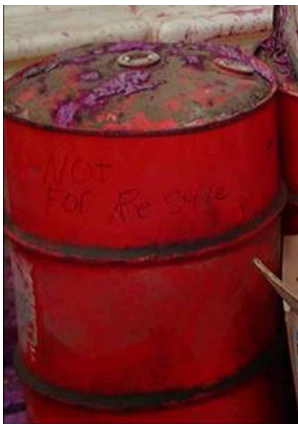
Figure 1. Pesticide drum bulging from extreme heat.
