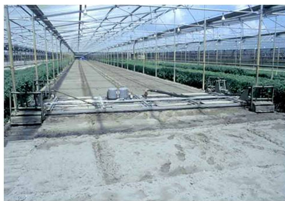
Figure 9. Mobile, winch drawn steam system to introduce steam directly under inverted pan to control nematodes and other soilborne pests in a greenhouse production system.
