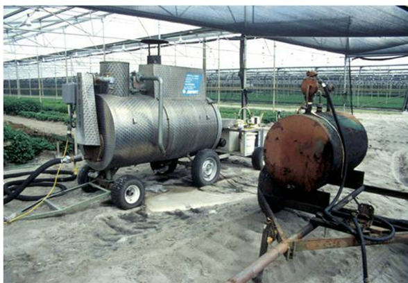
Figure 8. Small portable steam boiler and diesel fuel supply tank.
