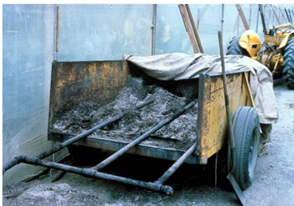
Figure 5. Small-scale system for introducing steam via a manifold of perforated pipe into a soil bin for nematode control in a greenhouse production system.
