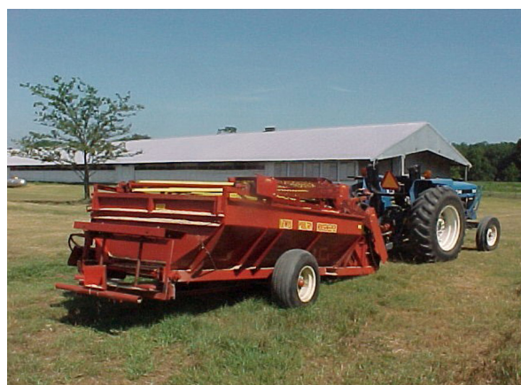
Figure 9. Manure spreader that can be used to apply manure for mulched vegetable crop production. Credits: J. Jones
