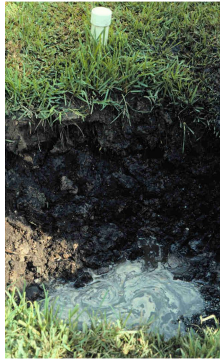
Figure 8. This planting site has a high water table, which is unsuitable for palm installation. Credits: Timothy K. Broschat
