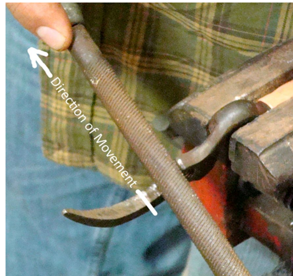
Figure 8. Using a round or half-round smooth file, file the edge of the curve perfectly flat. It is critical that you file this edge at 90° to the inside of the blade. Again, move the file in only one direction and avoid short, jerky strokes. Credits: G.C. Denny
