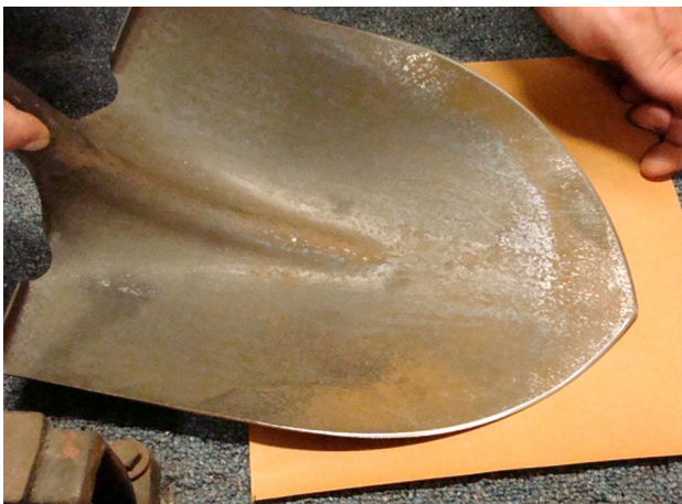
Figure 4. Use 300-grit sandpaper to remove any burrs on the back side of the blade. Credits: G.C. Denny
