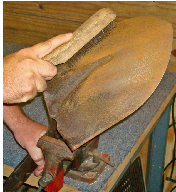
Figure 2. Use a wire brush to remove rust and debris. Credits: G.C. Denny
