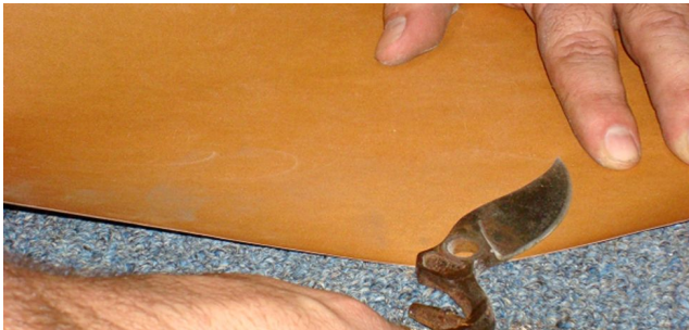
Figure 7. Use 300-grit sandpaper to remove any burrs on the back side of the blade. Credits: G.C. Denny
