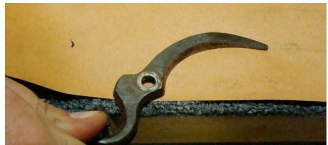
Figure 9. Use 300-grit sandpaper to remove any burrs on the back side of the blade. Credits: G.C. Denny
