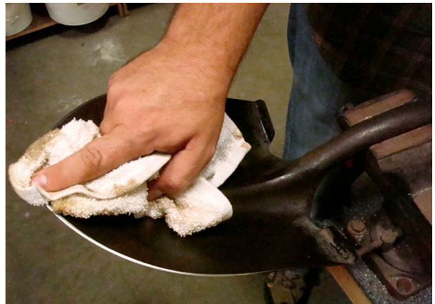
Figure 5. Wipe a thin layer of oil on the blade of the shovel to prevent rust. Credits: G.C. Denny
