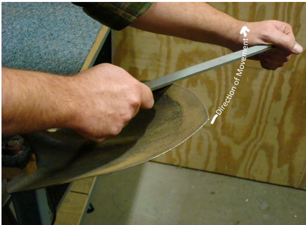
Figure 3. Move the file in only one direction and avoid short, jerky strokes. Credits: G.C. Denny
