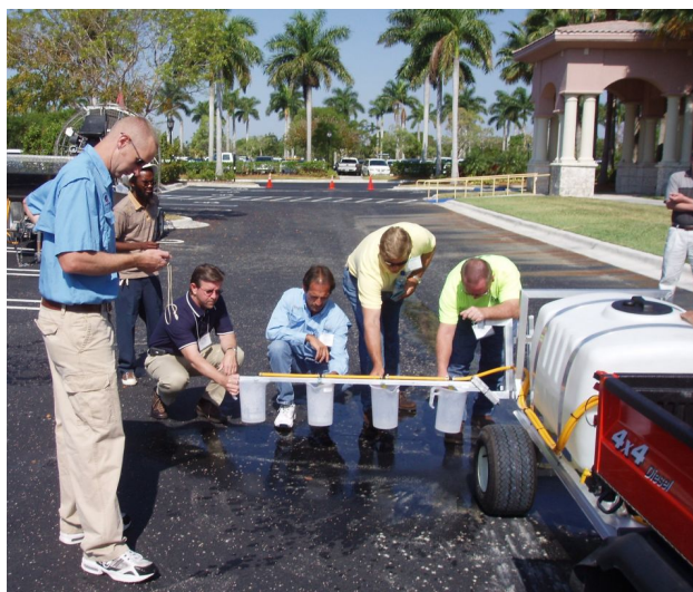
Figure 4. Checking a sprayer's output to determine the amount applied. Credits: F.M. Fishel, UF/IFAS PIO.
