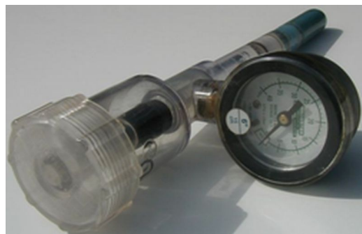
Figure 2. Tensiometer before being installed in the field. Credits: Harry Trafford
