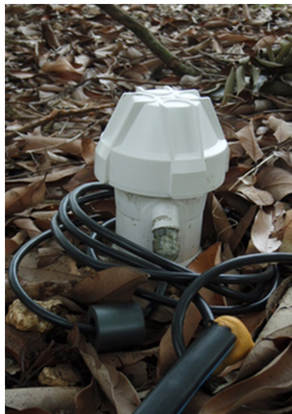
Figure 5. Multi-sensor capacitance probe installed in a south Florida grove. Credits: Luis Barquin
