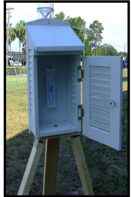
The weather shelter should be mounted on either a post or tripod, and ideally placed on a natural surface in an open area away from trees and buildings. This minimizes the influence of man-made objects on the temperature and rainfall. The opening of the shelter should also face away from the equator, or toward the north to minimize the effects of direct sunlight on the thermometer.
