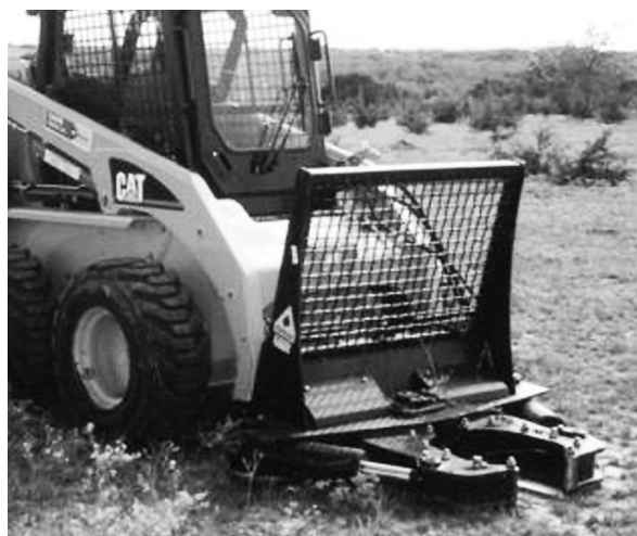
Figure 6. Modifications to small excavators, like the addition of this feller to cut trees, make them useful in interface forest harvesting. Credits: Photo courtesy of Virginia Tech
