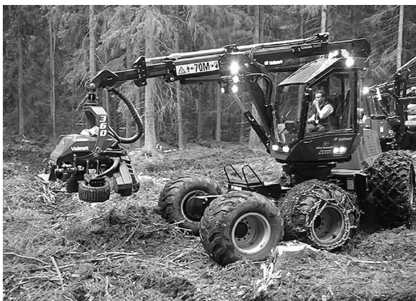
Figure 9. Modern telescoping boom harvester, with a processing head. Note tire chains for wet weather and soil protection. Credits: Photo courtesy of Virginia Tech.
