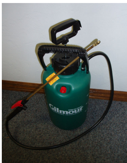
Figure 2. Handheld compression sprayer with a 2-gallon capacity.
