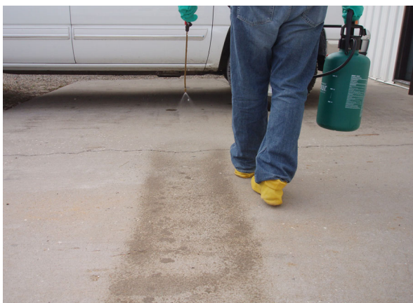
Figure 7. Checking the output of a compression sprayer.
