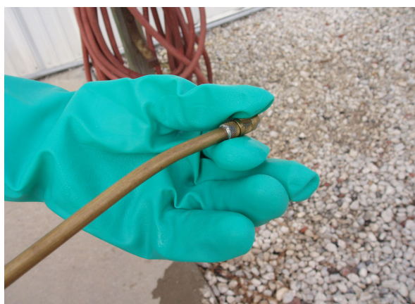
Figure 3. The nozzle tip can be rotated to adjust the delivery.
