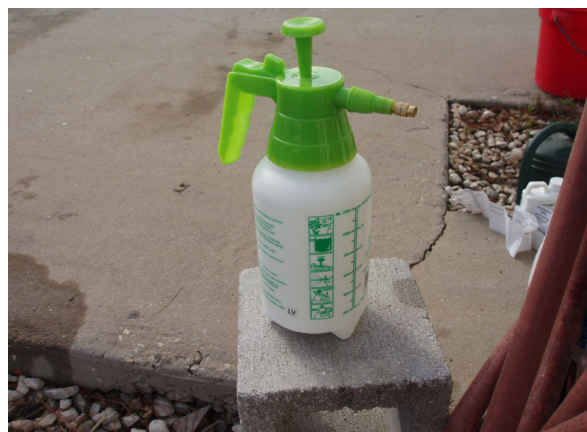
Figure 1. Handheld compression sprayer with a 44-ounce capacity.
