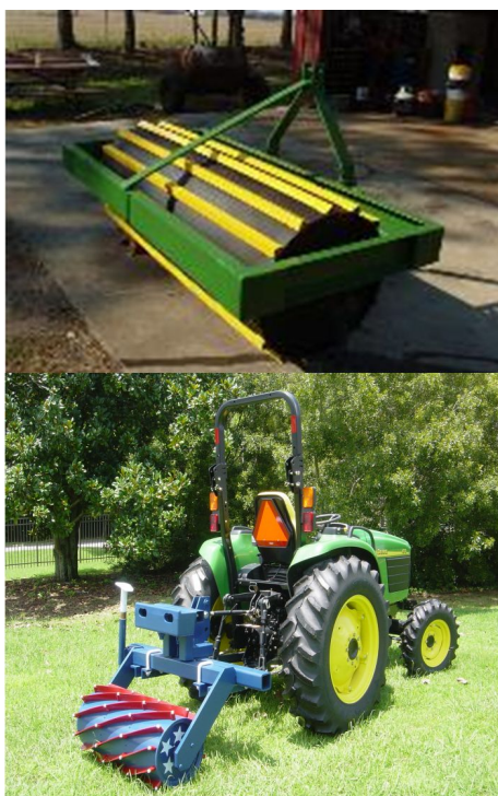
Figure 4. Roller-crimpers designed to terminate cover crops for reduced tillage systems. Top: Roller-crimper designed by D. Treadwell and M. Alligood, Horticultural Sciences Department, University of Florida 2006. Bottom: Roller-crimper designed by R. Raper, USDA-ARS-NSDL Conservation Systems Research, Auburn, AL Credits: Top: D Treadwell. Bottom: R. Raper
