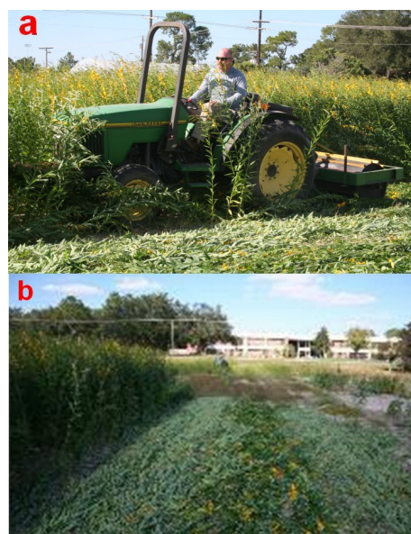
Figure 3. A) Roller-crimper designed by Alligood and Treadwell, terminating sunn hemp in Gainesville, FL, at mid-bloom. B) Terminated sunn hemp immediately following rolling and crimping Credits: D. Treadwell
