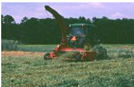
Figure 2. Flail chopper mowing a winter cover crop of annual hairy vetch and rye Credits: D. Treadwell
