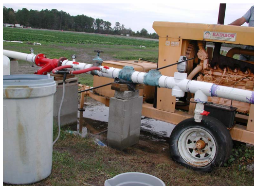
Figure 2. Diesel engines mounted on a trailer offer the greatest flexibility of use. Credits: Eric Simonne.
