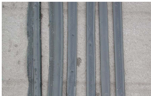
Figure 3. Drip tapes can be distinguished and recognized by their features. Note the emitter (on the four tapes on the right) and the turbulent flow channels (on the two tapes on the left). Credits: Eric Simonne.
