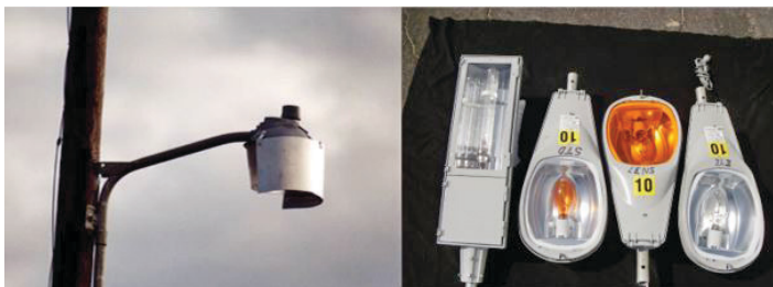
Figure 2. Light fixtures shielded on the top and sides direct light downward to reduce the likelihood of disorienting turtles on the beach (left). Examples of types of bulbs less likely to disorient turtles are (from left to right) low-pressure sodium vapor light, high-pressure sodium vapor fixture with specially coated amber high-pressure sodium vapor bulb (Eye Lighting International), high-pressure sodium vapor fixture and bulb with amber lens, and for comparison, a stock high-pressure sodium fixture and bulb. All except the fixture on the far right produce longer-wavelength light (>560 nm) which is less attractive to turtles.
