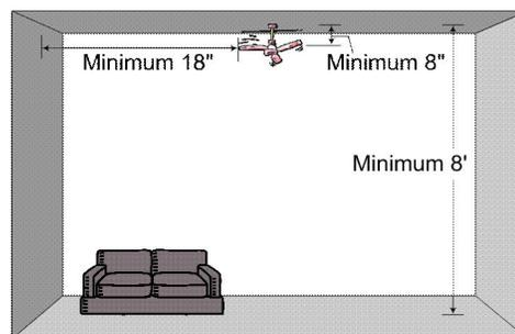
**Figure 1.** Minimum space requirements for a ceiling fan installation recommended by the U.S. Department of Energy. Credits: Image created by Hyun-Jeong Lee in Microsoft Office Visio. Converted to .GIF by IFAS Communication Services.
