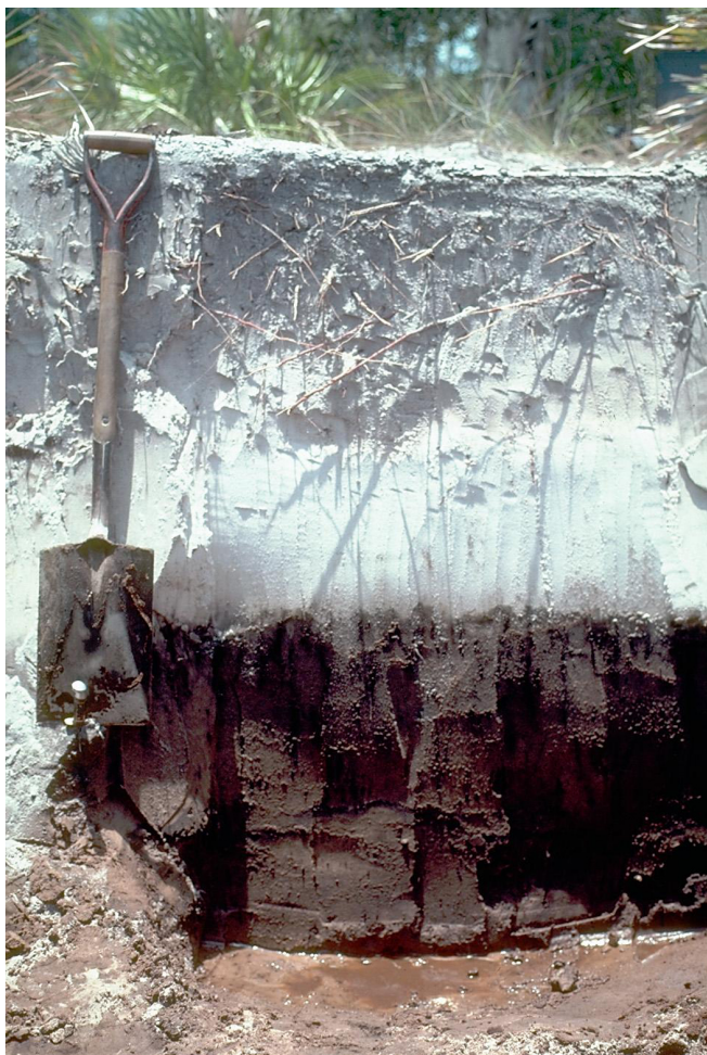
Figure 7. This Immokalee fine sand has the typical profile of a Spodosol. Note the dark stained layer, the spodic horizon, in the lower portion of the picture caused by a buildup of iron, aluminum, and organic matter (Source: Obreza et al., 2006).
