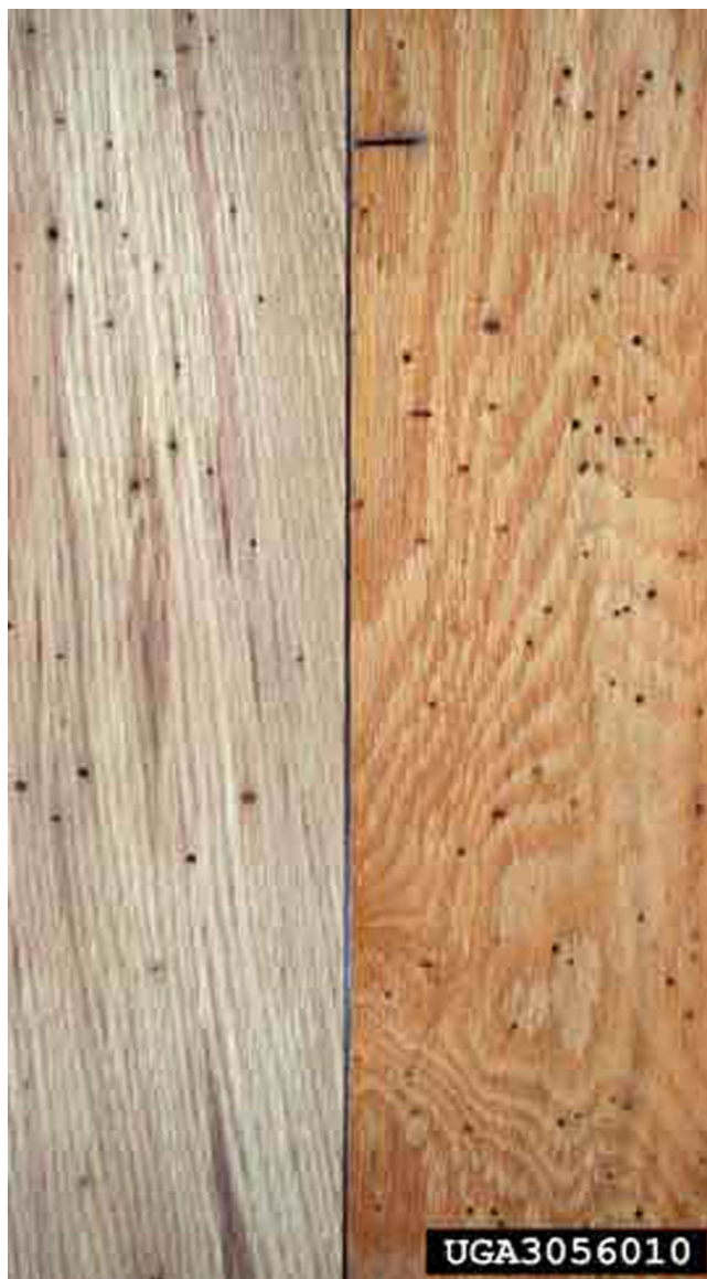
Figure 4. Damage (holes) caused by oak timberworm, Arrhenodes minutus (Drury), a primitive weevil. Credits: James, Solomon, USDA Forest Service; www.forestryimages.org
